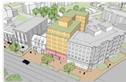
OP model for a 65-foot-high addition atop the former Yenching Palace restaurant building, immediately to the right of the historic firehouse. There is no setback until the top floor. DC Office of Planning.
