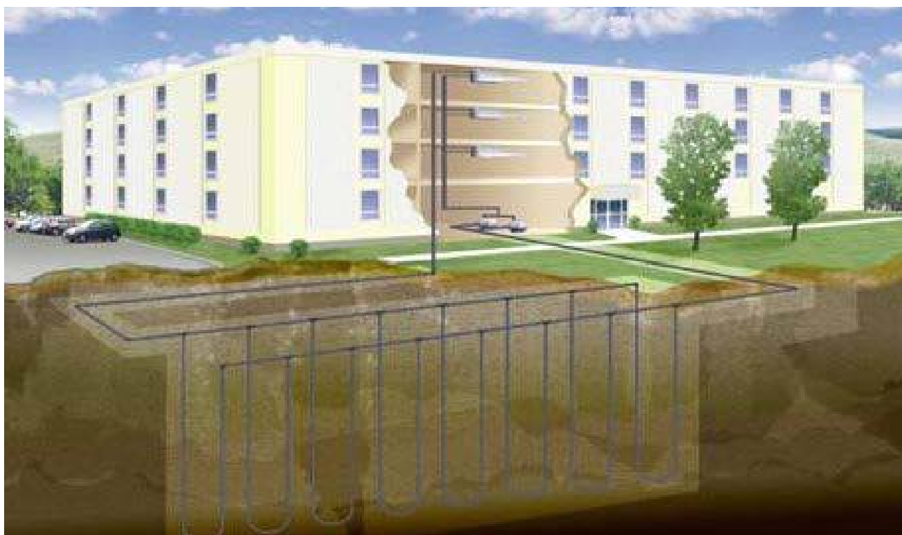
DIAGRAM OF A TYPICAL VERTICAL, CLOSED-LOOP SYSTEM
