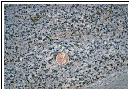
Salt and pepper texture of the Kensington Tonalite (aka Rock Creek granite), as seen in a specimen from the former Newark Street quarry. Many structures in Cleveland Park are faced with this classic building stone. Photo by Tony Fleming
